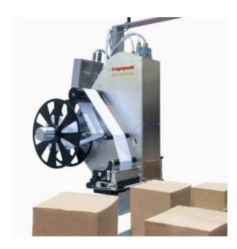
**Eco-Labeller, Logopak's**new labelling machine, is also giving up the support for silicon paper labels. Compared to a conventional automatic labeler, the running time is extended by 50% thanks to a longer consumable coil. The label is printed and cut to the desired format without limitation. The adhesive can be pre-activated or the activation is done on demand. It offers a high printing speed, up to 300 mm/s.
